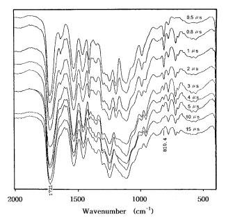
**Figure 2** The changes in IR spectra of photocurable acrylic resin with the exposure of argon ion laser.
