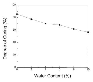
**Figure 5** The effect of water as a viscosity reducer on the curing velocity of resin: laser power (1 W), exposure time (4  $\mu$ s), IRR 160 (93 wt %), and D 184 (7 wt %).
