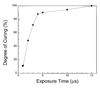
**Figure 3** Dependence of the laser-curing degree on exposure time: laser power (1 W), IRR 160 (90%), and D 184 (10%).
