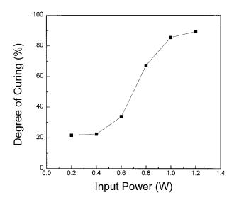
**Figure 4** Dependence of the laser-curing degree on the input power of the laser: exposure time  $(4 \ \mu s)$ , IRR 160 (93 wt %), and D 184 (7 wt %).
